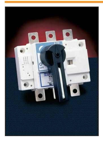
The Ferraz Shawmut Surge Switch is an extremely compact, high performance, manually operated, non-fused switch. It is specifically designed to withstand the high surge current of 200kA with an 8x20  $\mu$ s waveform seen in today's transient voltage surge protection device (SPD) applications. Ferraz Shawmut's Surge Switch utilizes a unique contact design that actually clamp contacts tighter during a surge.
